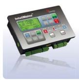
InteliMains<sup>NT</sup> is designed for multiple (up to 31) gen-sets operating in parallel to mains. InteliMains controller connects the group of gen-sets to the mains. It can serve as a bus-tie synchronizing controller between two groups of gen-sets.
