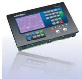
InteliSys<sup>NT</sup> is an expandable controller for both single and multiple gen-sets operating in standby or parallel modes, especially in CHP and other complex applications. Detachable construction (consisting of IS-NT-BB and IS-Display or InteliVision) allows easy installation with the potential for many different extension modules designed to suit individual customer requirements.
