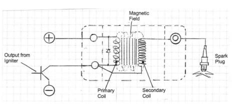
Then, having been pre-programmed, the igniter abruptly dumps the primary energy at the most optimum time to ground, i.e.the magnetic field collapses, and generates in the very high number of windings in the secondary coil a high tension voltage of over 25 Kilovolts, which creates at the spark plug a spark of a determined duration, resulting in optimum combustion and performance at lowest possible emission.
